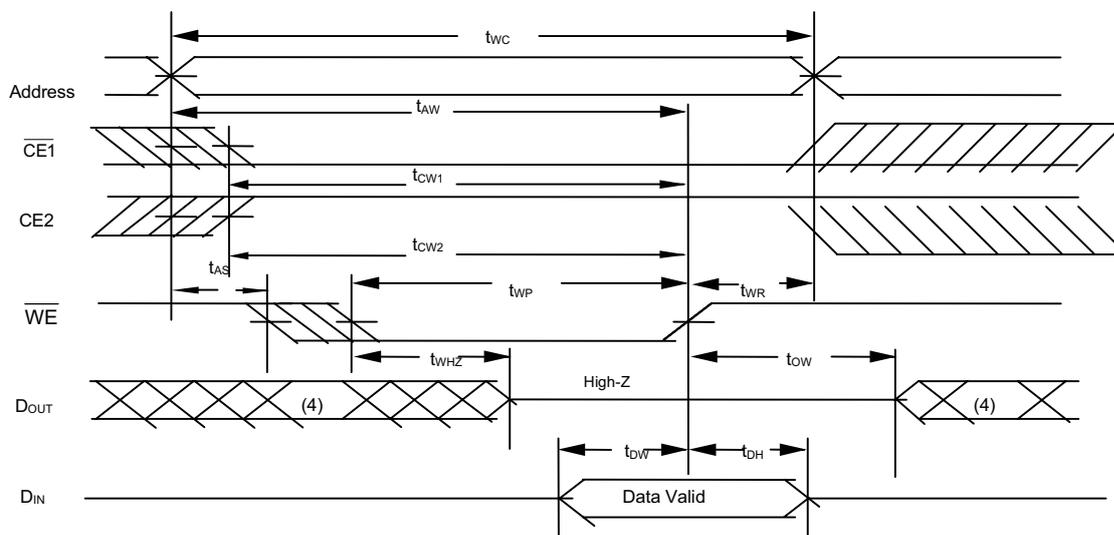
WRITE CYCLE 2 ( $\overline{CE1}$  and  $\overline{CE2}$  Controlled) (1,2,5)
