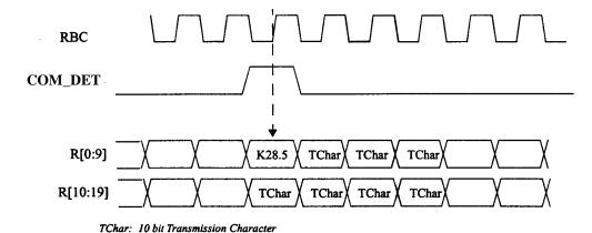
Figure 3. Detection of a Properly Aligned Comma Character
