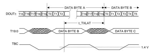
Figure 6. Transmitter Latency
