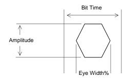
Figure 10. Receiver Input Eye Jitter Tolerance Mask Diagram
