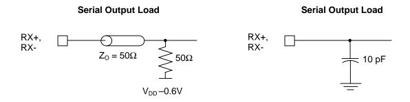
Figure 11. Parametric Test Load Circuit
