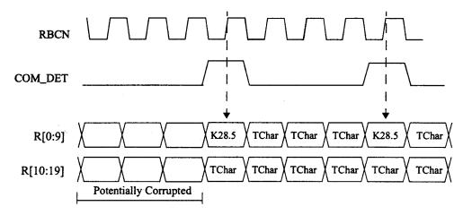
Figure 4. Detection and Resynchronization of an Improperly Aligned Comma Character
