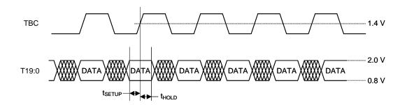
Figure 5. Transmitter Section Timing
