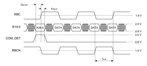
Figure 7. Receiver Section Timing
