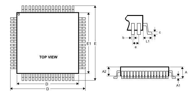
Figure 7. Mechanical Dimensions
