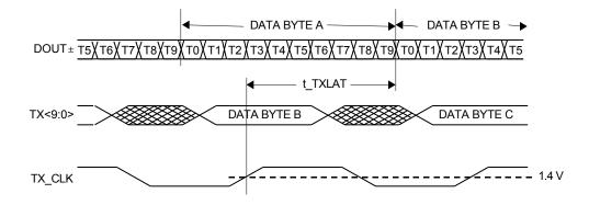
Figure 4. Transmitter Latency
