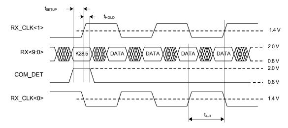
Figure 5. Receiver Section Timing
