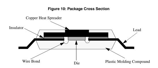
The thermal resistance for the VSC8116 package is improved through low thermal resistance paths from the die to the exposed surface of the heat spreader and from the die to the lead frame through the heat spreader overlap of the lead frame.
