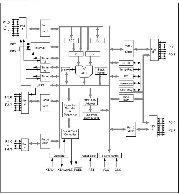
Figure 2. Architecture of the W78C54
