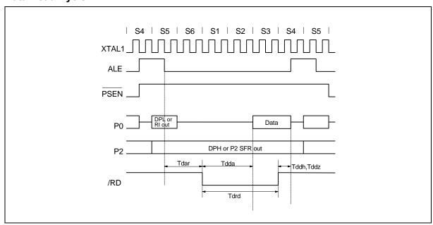
Figure7. External Data Memory Read Cycle
