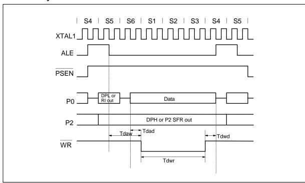
Figure 8. External Data Memory Write Cycle
