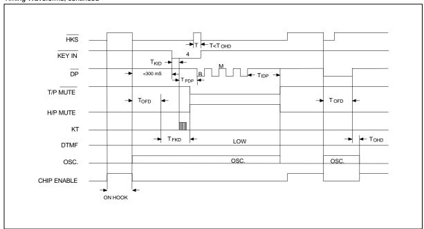
Figure 4 Lock Function Timing Diagram
