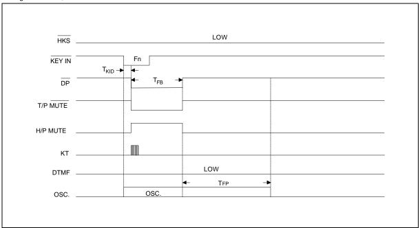
Figure 8 Flash Operation Timing Diagram
