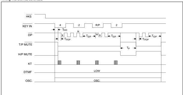
Figure 6 Pause Function Timing Diagram (without lock)
