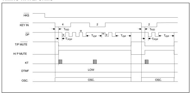
Figure 1(a) Pulse Mode Tming Diagram (Normal dialing without lock function)
