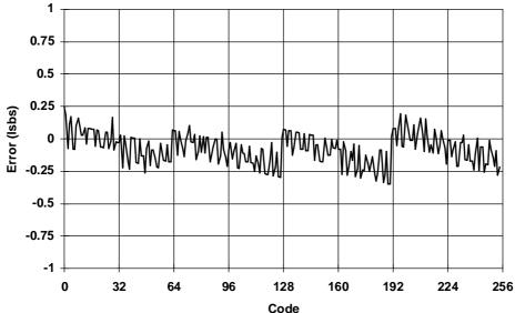
Test conditions: Vcc = 5V. VREF = 5V, Temp = 25°C, Fclk = 250KHz
