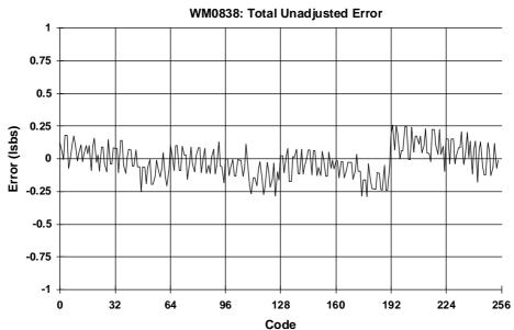
Test conditions: VDD = 5V, VREF = 5V, Temp = 25°C, FCLK = 250kHz
