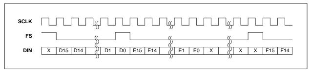
Figure 8 Interface Timing in DSP Mode
