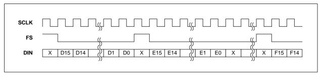
Figure 7 Interface Timing in Microcontroller Mode
