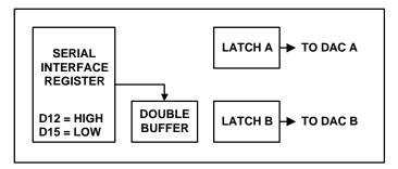
Figure 9 Double Buffer Only Write
