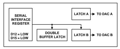
Figure 8 Latch B and Double Buffer Write
