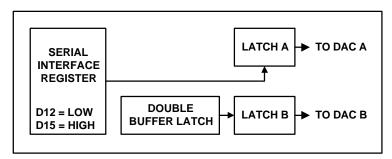
Figure 7 Latch A Write, Latch B Update
