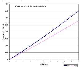
Figure 3 Sink Current VDD = 3V
