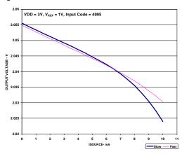
Figure 5 Source Current VDD = 3V
