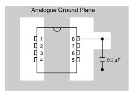
Figure 5 - Power-Supply Bypassing
