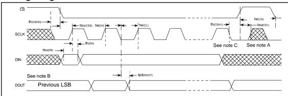
NOTES: A. The input clock, applied at the SCLK terminal, should be inhibited low when CS is high to minimise clock feedthrough. B. Data input from preceding conversion cycle.
