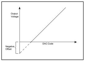
Figure 4 - Effect of Negative Offset (Single Supply)
