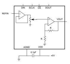
Figure 1 - Typical Operating Circuit
