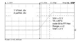
Rise time = 2.4  $\mu$ s, Positive slew rate = 1.0  $\mu$ s Settling time = 5.8  $\mu$ s
