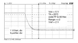
Fall time = 5.0  $\mu$ s, Negative slew rate = 0.63  $\mu$ s Settling time = 9.5  $\mu$ s
