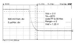
Fall time = 4.25  $\mu$ s, Negative slew rate = 0.46  $\mu$ s Settling time = 8.5  $\mu$ s
