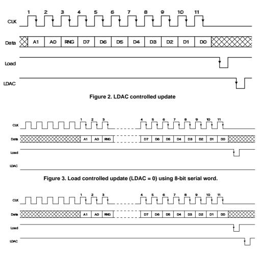
Figure 4. LDAC controlled update using 8-bit serial word.
