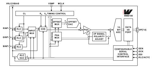
Figure 16 Signal Path When in Line-by-Line Mode
