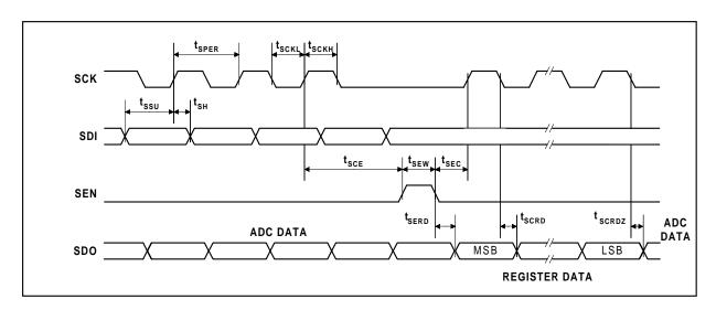
Figure 4 Serial Interface Timing
