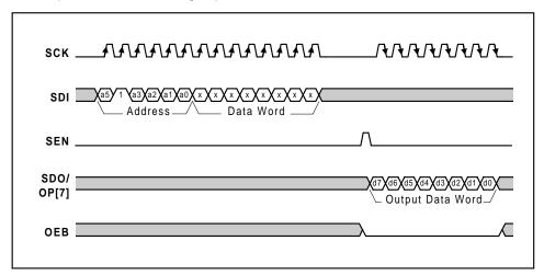
Figure 14 Serial Interface Register Read-back
