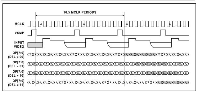
Figure 21 Mode 5 Operation (MCLK:VSMP Ratio = 8:1)
