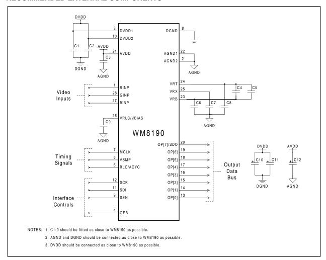
Figure 23 External Components Diagram
