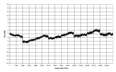
Figure 6 INL Vs Output Data Codes
