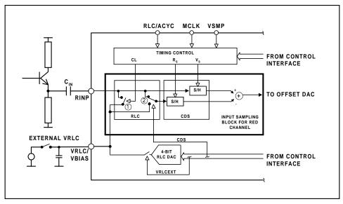
Figure 7 Reset Level Clamping and CDS Circuitry
