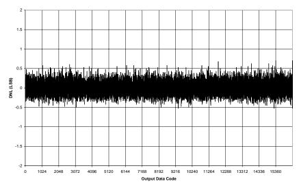
Figure 5 DNL Vs Output Data Codes
