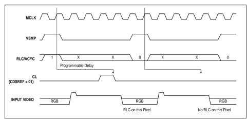
Figure 8 Relationship of RLC Pin, MCLK and VSMP to Internal Clamp Pulse, CL
