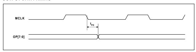
Figure 2 Output Data Timing
