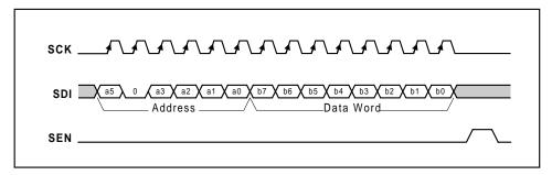
Figure 13 Serial Interface Register Write
