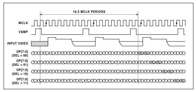
Figure 22 Mode 6 Operation (MCLK:VSMP Ratio = 8:1)
