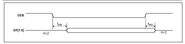
Figure 3 Output Data Enable Timing
