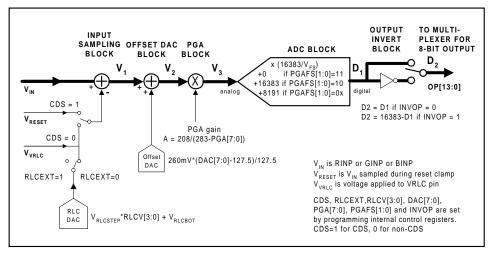
Figure 10 Overall Signal Flow
