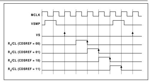
Figure 9 Reset Sample and Clamp Timing
