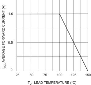
T<sub>L</sub>, LEAD TEMPERATURE (°C) Fig. 1 Forward Current Derating Curve
