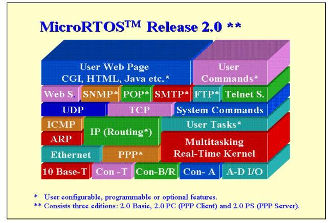
The Slim-Link<sup>®</sup> Server operates with MicroRTOS<sup>TM</sup>, Multi-User, Multi-Task Real-Time Operating System. This operating system permits the Slim-Link Server to support multiple users and to run multiple tasks simultaneously in real-time. Multiple users can be connected to either serial port or over the ethernet connection to the HTTP server.
