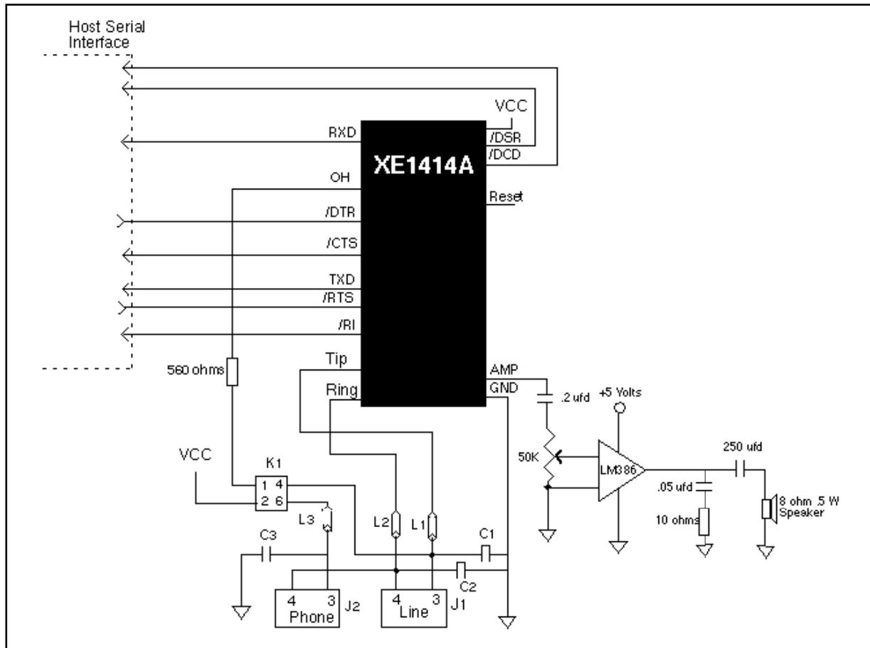
Note: RJ11 Pin assignments reflect a 6-pin connector. Tip and Ring are always the center pins of the RJ11 jack.
