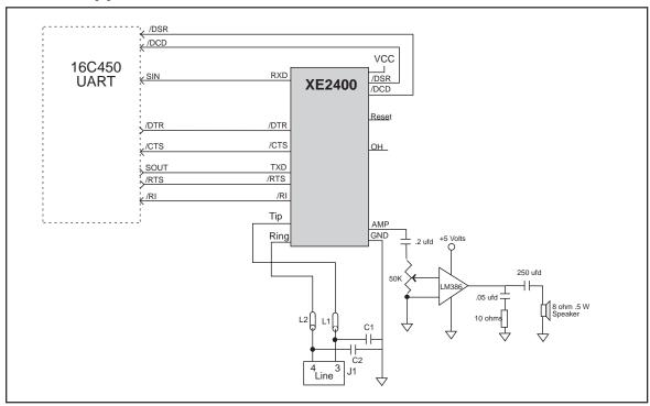
Note: RJ11 Pin assignments reflect a 6-pin connector. Tip and Ring are always the center pins of the RJ11 jack.
