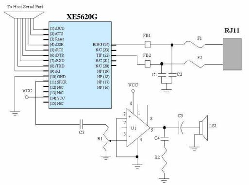
Parts List for XE5620G Typical Connection Diagram
