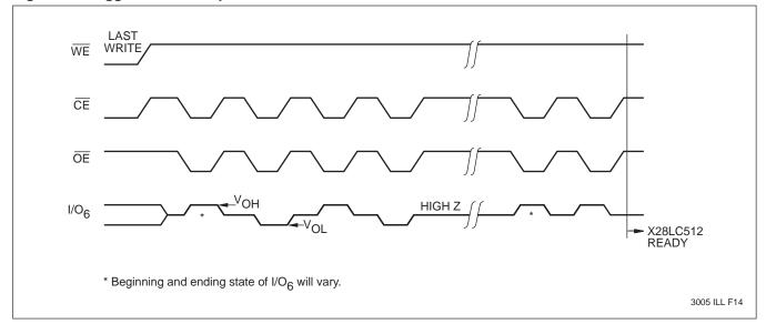
The Toggle Bit I/O<sub>6</sub> Figure 3a. Toggle Bit Bus Sequence
