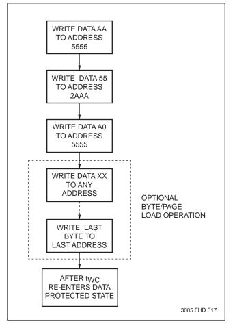
Regardless of whether the device has previously been protected or not, once the software data protected algorithm is used and data has been written, the X28LC512/513 will automatically disable further writes unless another command is issued to cancel it. If no further commands are issued the X28LC512/513 will be write protected during power-down and after any subsequent power-up. The state of  $A_{15}$  while executing the algorithm is don't care.
