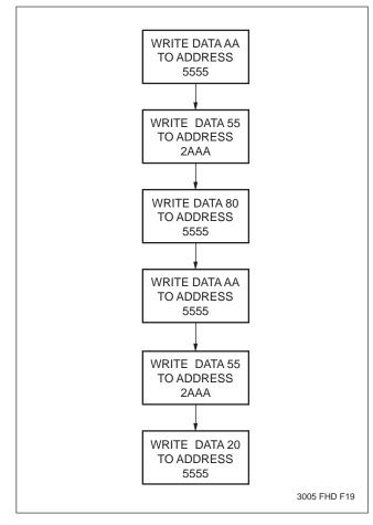
In the event the user wants to deactivate the software data protection feature for testing or reprogramming in an E<sup>2</sup>PROM programmer, the following six step algorithm will reset the internal protection circuit. After t<sub>WC</sub>, the X28LC512/513 will be in standard operating mode.
