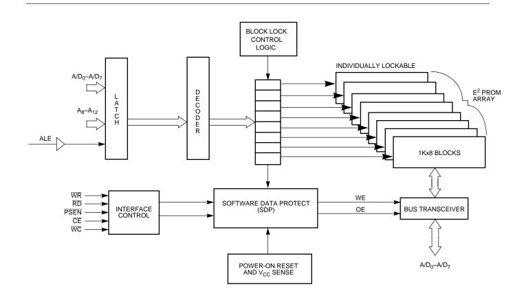
Software Data Program Control provides a lower level of memory write management. SDP controls write operations to the entire memory. When enabled, the host microprocessor must send a special 3 byte command sequence before any byte or page writes to unlocked locations in the memory.
