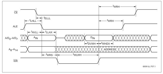
Note: (7) t<sub>WC</sub> is the minimum cycle time to be allowed from the system perspective unless polling techniques are used. It is the maximum time the device requires to automatically complete the internal write operation.
