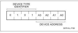
The next four bits of the slave address are the device address. The physical device address is defined by the state of the A0-A3 inputs. The X9221 compares the serial data stream with the address input state; a successful compare of all four address bits is required for the X9221 to respond with an acknowledge.
