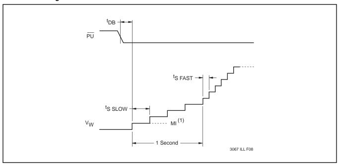
Notes: (1) MI in the A.C. timing diagram refers to the minimum incremental change in the wiper voltage.
