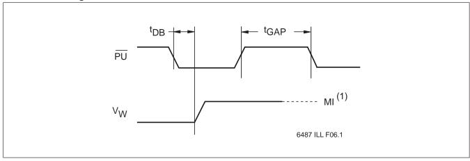
Notes: (1) MI in the A.C. timing diagram refers to the minimum incremental change in the wiper voltage.
