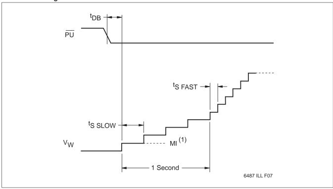
Notes: (1) MI in the A.C. timing diagram refers to the minimum incremental change in the wiper voltage.
