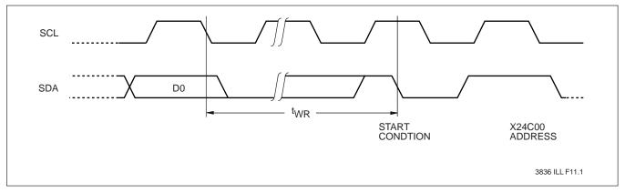
Note: (4) The write cycle time is the time from the initiation of a write sequence to the end of the internal erase/program cycle. During the write cycle, the X24C00 bus interface circuits are disabled, SDA is high impedance, and the device does not respond to start conditions.
