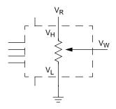
Three terminal potentiometer; variable voltage divider
