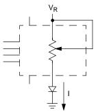
Two terminal variable resistor; variable current
