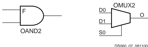
Figure 7: AND and MUX Symbols in Spartan-XL IOB
