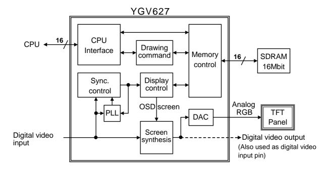
YGV627 is connected to the external memory bus of CPU as an external I/O device. As a video memory, SDRAM of up to 64M bits can be connected to local memory bus of YGV627 to send bitmap image data stored in the video memory into monitor as RGB signal in accordance with display scan timing.
