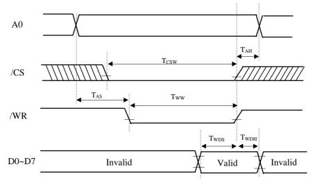
Note:  $T_{CSW}$ ,  $T_{WW}$ ,  $T_{WDH}$  and  $T_{AH}$  are defined with respect to the moment /CS or /WR becomes High level.
