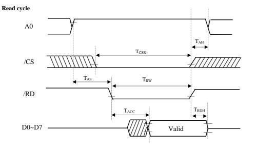
Note:  $T_{ACC}$  is defined with respect to the moment /CS or /RD becomes Low level later.  $T_{CSR}$ ,  $T_{RW}$ ,  $T_{RDH}$  and  $T_{AH}$  are defined with respect to the moment /CS or /RD becomes High level.
