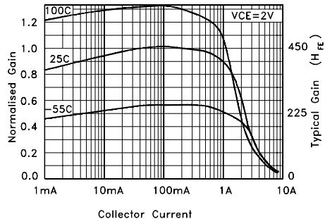
FIG. 3  $H_{FE}$  vs  $I_C$
