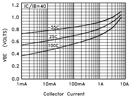
FIG. 4  $V_{BE(SAT)}$  vs  $I_C$
