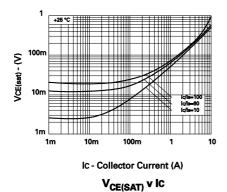
The Zetex FMMT617 is an ideal choice of transistor, having a low saturation voltage. A data sheet for the FMMT617 is available on Zetex web site or through your local Zetex sales office. Outline information is included in the characteristics section of this data sheet.
