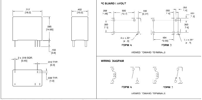
Dimensions in inches with metric equivalents in parentheses. Tolerance: ± .010"
