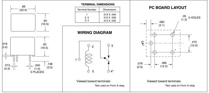
Dimensions in inches with metric equivalents in parentheses. Tolerance: ±0.010"
