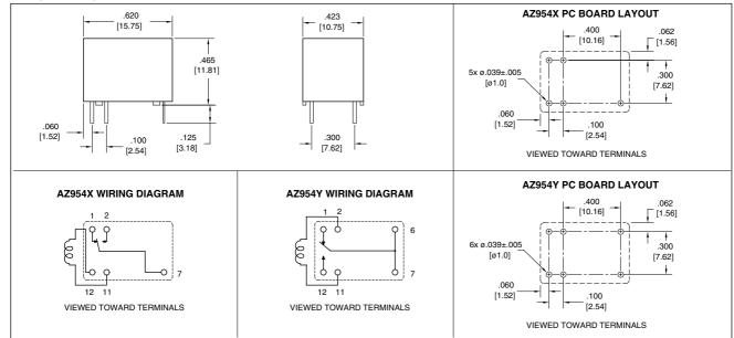
Dimensions in inches with metric equivalents in parentheses. Tolerance:  $\pm 0.010"$
