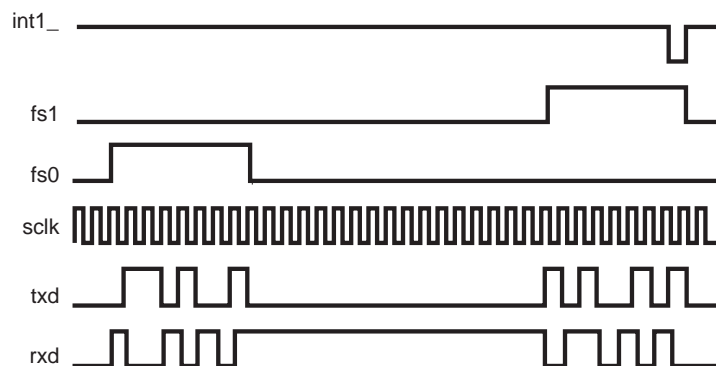
Figure 21. CODEC Interface Timing (8-Bit Mode)
