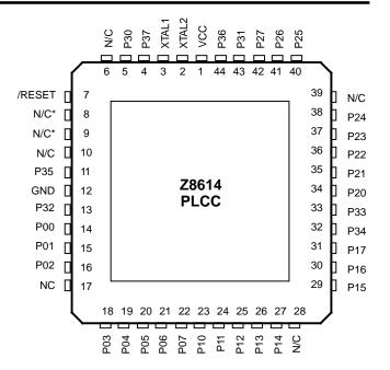
Note: Pins 8 and 9 actually are connected to the chip, although used only for testing. These pins must be used as floaters by the customer.
