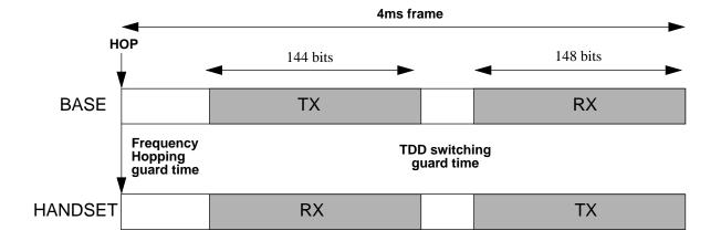
Figure 1. Basic Time Duplex Timing
