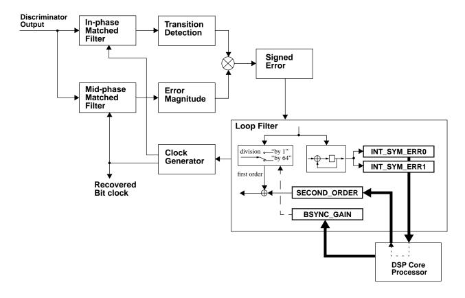
Figure 6. Bit Synchronizer Loop and Processor Control
