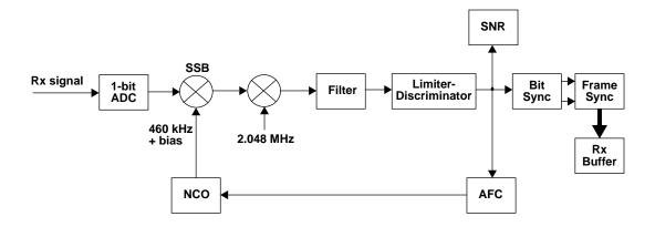
Figure 2. Demodulator Block Diagram
