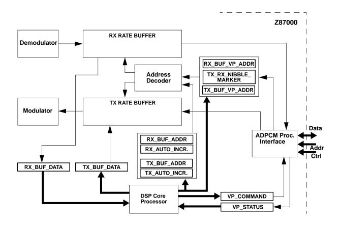
Figure 9. Rate Buffers Access and ADPCM Processor Interface
