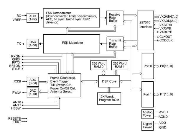
Figure 2. Z87000 Functional Block Diagram
