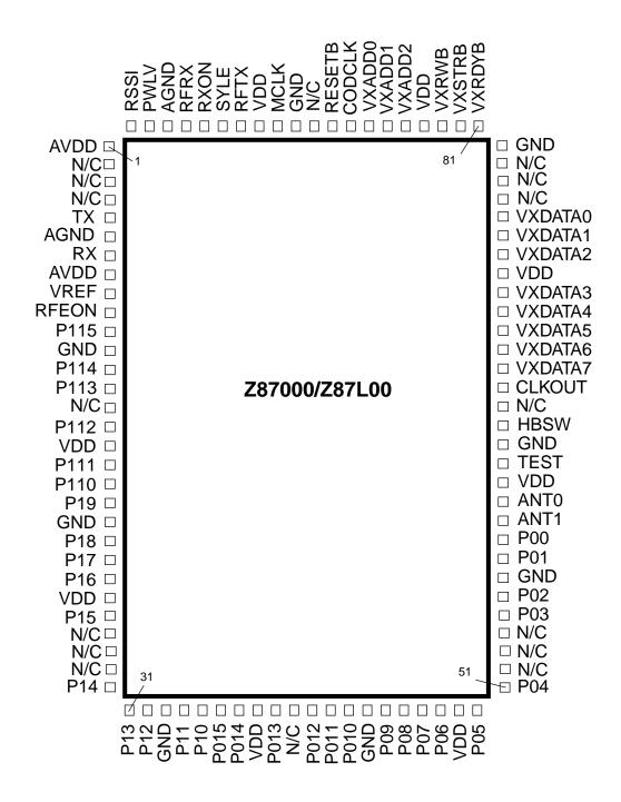
Figure 4. 100-Pin QFP Pin Configuration
