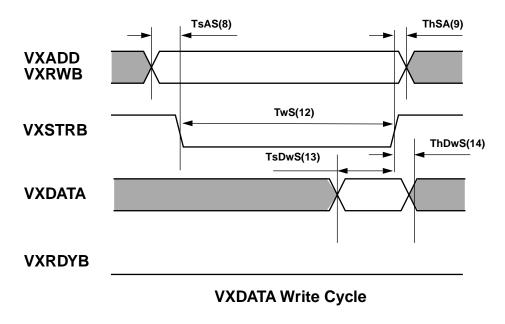
Figure 8. Read/Write Cycle Tlmings
