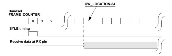
Figure 7. Frame Counter and UW LOCATION on Handset
