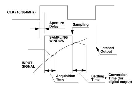
Figure 6. 1-Bit ADC Definition of Terms
