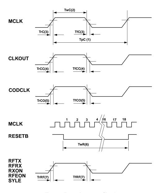
Figure 7. Transceiver Output Signal
