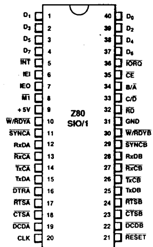
Figure 4. 40-pin Dual-In-Line Package (DIP), Pin Assignments
